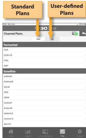
The standard plans can be cloned. When the user does this, a new channel plan is added to the User channel plans list:
