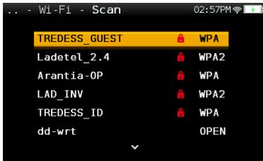
As you can see in the image above, the list shows the name of the Wi-Fi networks and indicates if the network is open or restricted, as well as the protection access type.
